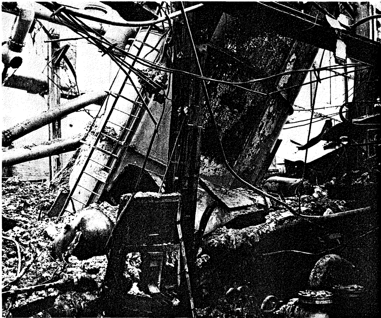
Figure 4. Position of upper section of the coldbox shell after the explosion.
